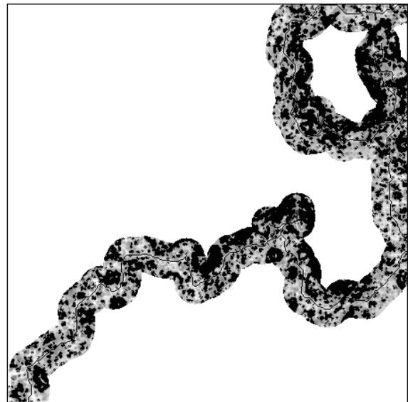
Figure 6 illustrates the same problem using coarse map information, created by averaging the arc costs in each square region. This map information is accurate enough to steer the robot to the correct side of the central obstruction, and the resultant path is only 6% greater in cost than omniscient optimal.
