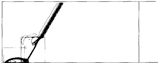
FIG. 6.1. Contour plot showing the effects of a strong shock passing through a grid boundary.
